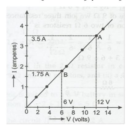
Resistance of resistor (R) =  $V_A - V_B / 1_A - 1_B = 12 \text{ V} - 6 \text{ V} / 3.6 \text{ A} - 1.8 \text{ A}$
