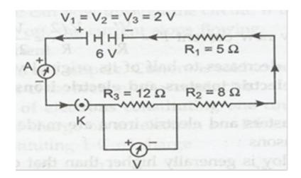
Here ammeter A has been joined in series of circuit and voltmeter V is joined in parallel to 12 ohms resistor.
